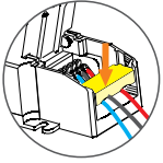
Push the wire pressing board to fix the wires.
